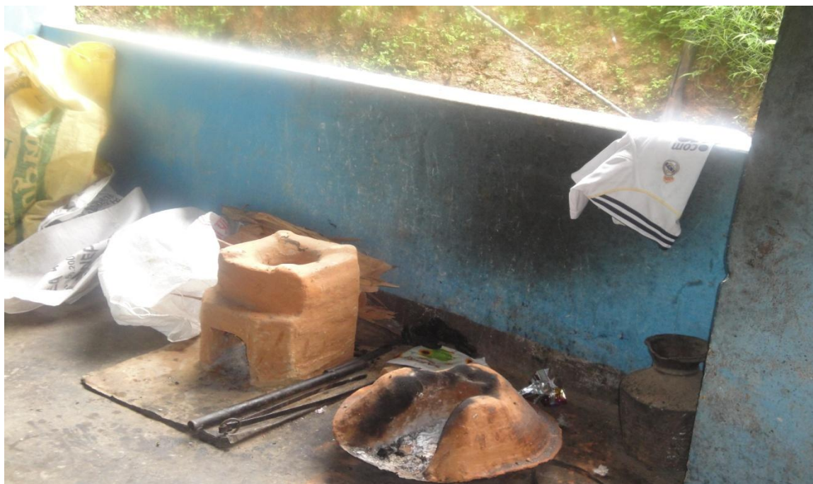
Figure 12. Rocket Stove along with Traditional Cook Stove
